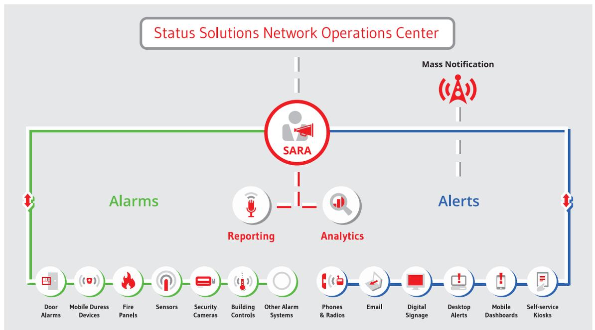
Architecture diagram of our Situational Awareness and Response Assistant (SARA) automated alerting engine, showing various alarm inputs and mass notification outputs customized to meet customer needs and infrastructure
